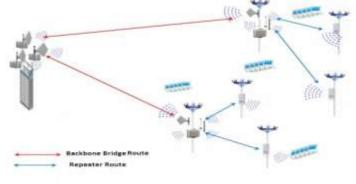
Figure 2: Mesh Architecture
