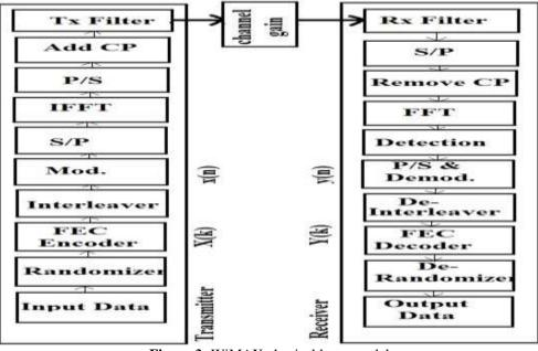
Figure 3: WiMAX physical layer model
